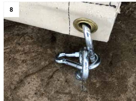
8. Hook the lower carabiner through eye-bolt in the floor anchor.
